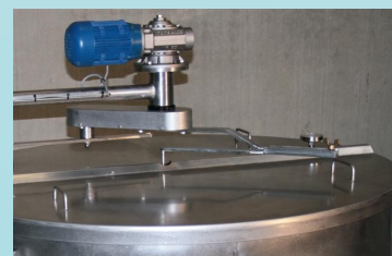
Stirring tool can be used with lids on the vat
